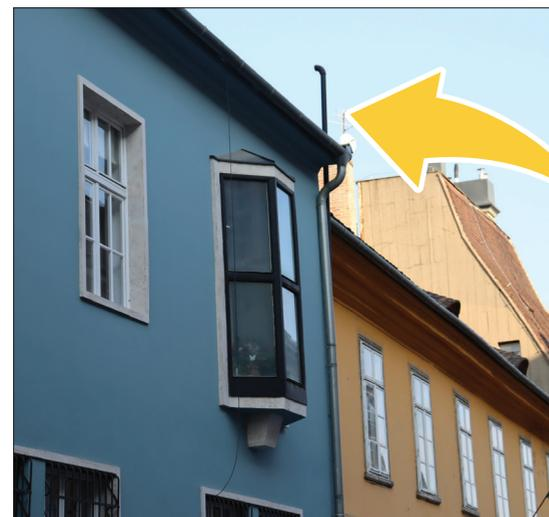
The mechanical part of the nuclear bunker was also connected to the surface at several points. Since these were also secret objects, they had to be disguised. The exhaust pipe, for example, was hidden behind the gutter of a house on Úri utca.
